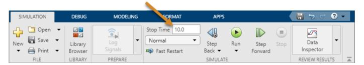
The default stop time of 10.0 is appropriate for this model. This time value has no unit. The time unit in Simulink depends on how the equations are constructed. This example simulates the
